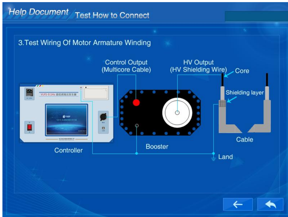
Figure 14 Wiring Diagram for Single-phase Cable Test
